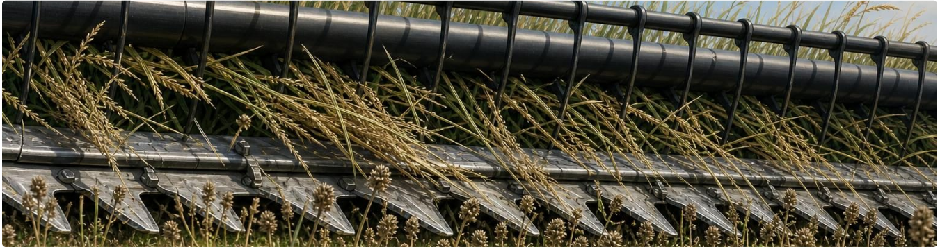
A harvester cuts tall grass seed heads while leaving shorter weed seed heads below the cutter.
